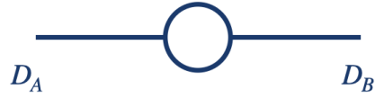
Figure 3.6: A single tensor with two dangling legs, each endowed with a Hilbert space of dimension D_A and D_B respectively.
